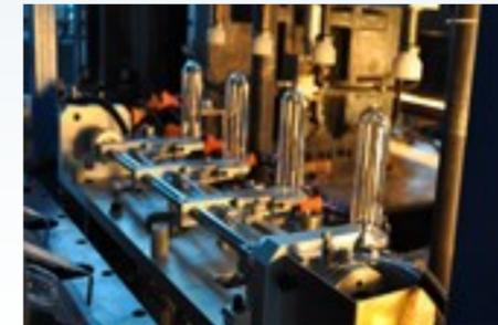
This machine's mold base adopts pressurized symmetry structural form of four formwork's back side, and has the advantages of fast motion, stability and reliability, small mechanical vibration. Opening and closing mold's power module adopts single power rotary connecting rod clamping mechanism.
